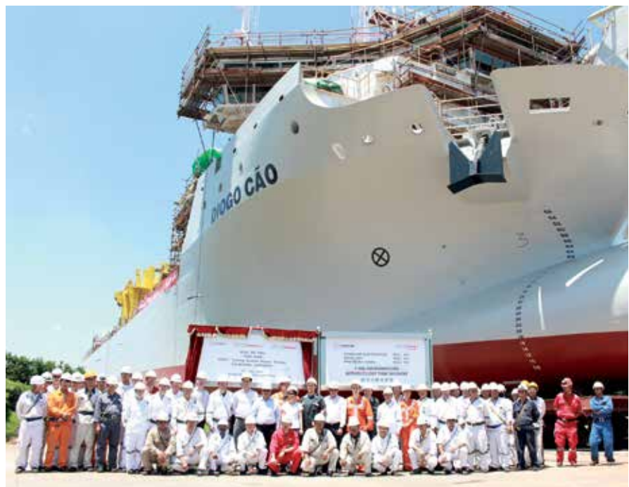
The 3,500m 3 TSHD launched in Keppel Nantong Shipyard, China, will be able to dredge to a maximum depth of 27.6m
