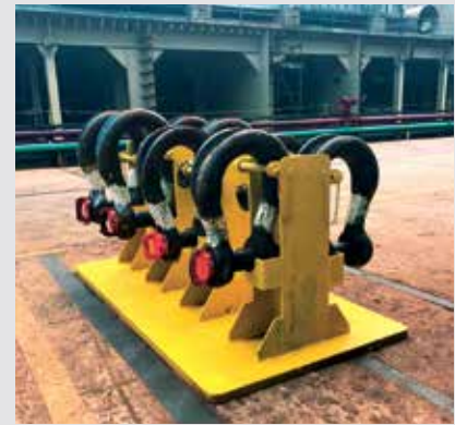
The innovative shackle jig drastically reduced the number of man-hours required for rigging and de-rigging jobs, resulting in significant cost savings
